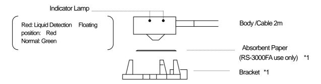
\*1: The Bracket is different for RS-3000FA and for RS-3000FAP. These differences are adsorbent paper use or not. For details, refer page 12 Specifications.
