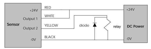
Note: The above wiring must be applied to the PNP Samples only.
