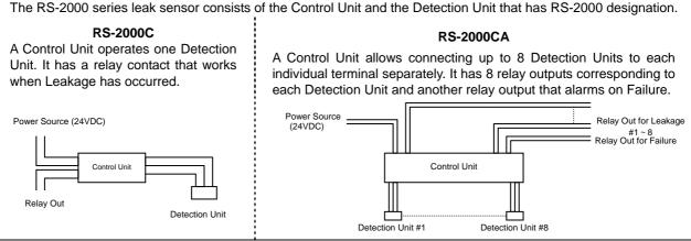
NOTE: The RS-2000 series control unit does not allow connecting 2 or more Detection Units to one terminal by parallel connection.
